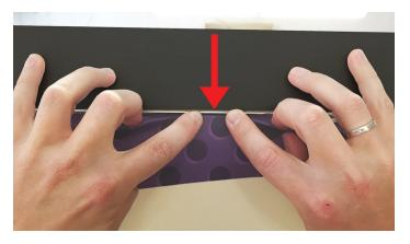
2 From the top center of the frame, insert the silicone gasket into the metal track.
