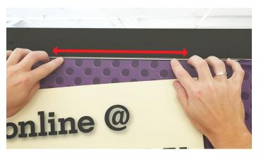
3 Using your index fingers, smooth outward towards the corners, guiding the silicone gasket into the metal track. Repeat this process for the bottom and both sides. Do not stretch the silicone gasket into place, it will not return to the original size.
