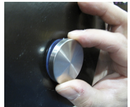
7 Tighten each cap until snug (do not over tighten).
