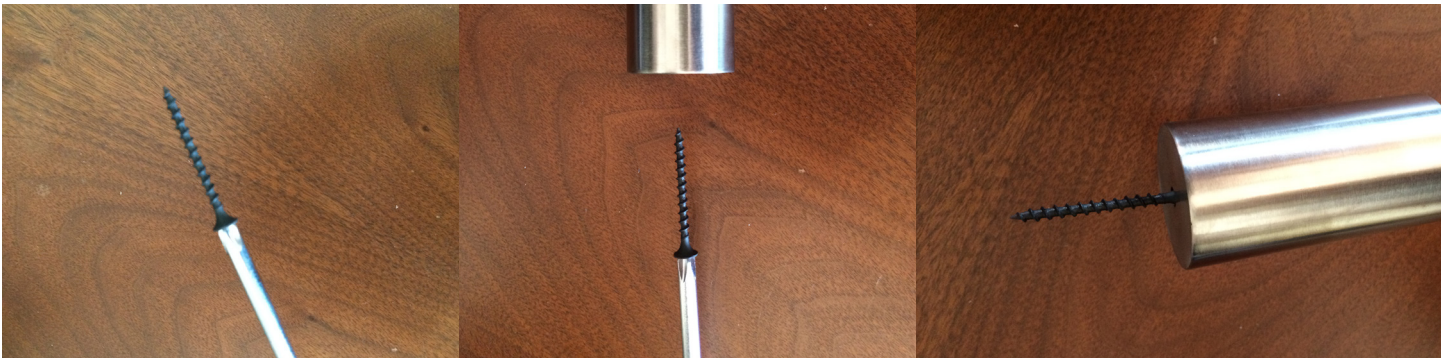
4 Using a long screwdriver extension, thread the screw through the barrel.
