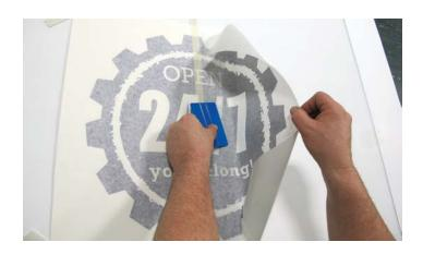
4. Now that half of the decal has been applied and it is fully anchored to the surface- you can now remove the remaining masking tape. Peel back the other half of the decal, remove the remaining backing liner, and apply the rest of the decal in the same manner.
