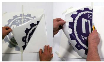
3. Hold the exposed decal just over the mounting surface making sure that it is taut. Start applying the decal from the center using the squeegee with firm overlapping strokes. The squeegee should be held at a 45 degree angle to prevent trapped air bubbles.
